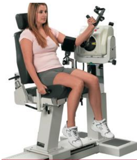
Figure 1: Isokinetic elbow arm flexion/ extension set up on Biodex.
