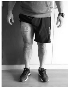
Figure 1: Placement of the measurement devices: activPAL on the middle-line of the right thigh (one third of the way between hip and knee) and Garmin watch on the left wrist.
