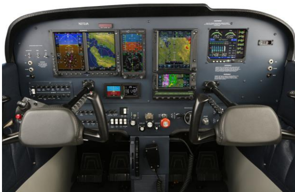
Figure 5: Retrofit Garmin G500 Glass cockpit – cockpit Cessna 172N (1979)
