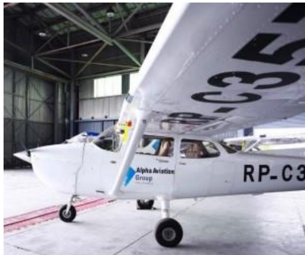
Figure 3: The Cessna 172, a four-seater, single-engine aircraft equipped with modern digital avionics (AAG)
