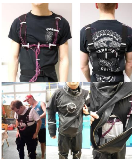
Figure 9: Prototype of vibrational interface for diver supporting systems, left wearing at torso of probands in a lab, right user tests in public swimming pool (under diving dry suit)
